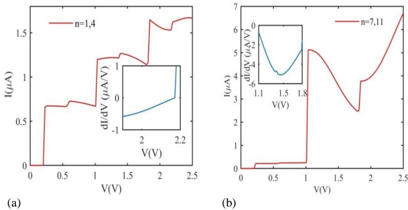
**Fig. 6.** (Colour on-line I-V characteristic when there are two Carbon atoms are substituted with Nitrogen atoms on (a)  $n=1, 4$  and (b)  $n=7,11$ .
