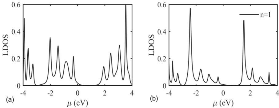
**Fig. 3.** Local density of states (LDOS) of the multi polythiophene molecular bridge versus energy of incoming electrons for polythiophene (a) without and (b) with Nitrogen atom on site  $n=1$ .
