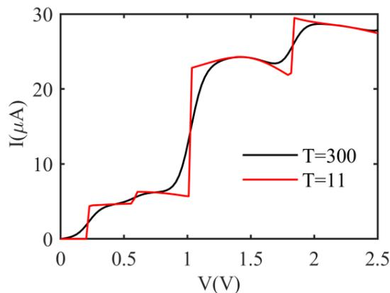
**Fig. 4.** (Colour on-line) I-V characteristics of polythiophene molecular bridge in  $T=11\text{K}$  and  $T=300\text{K}$ .
