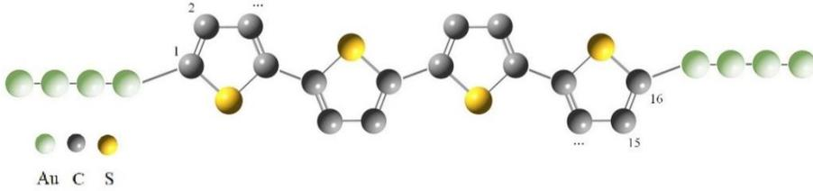
**Fig. 1.** (Colour on-line). Scheme diagram of the structure of a polythiophene sandwiched between metal leads.
