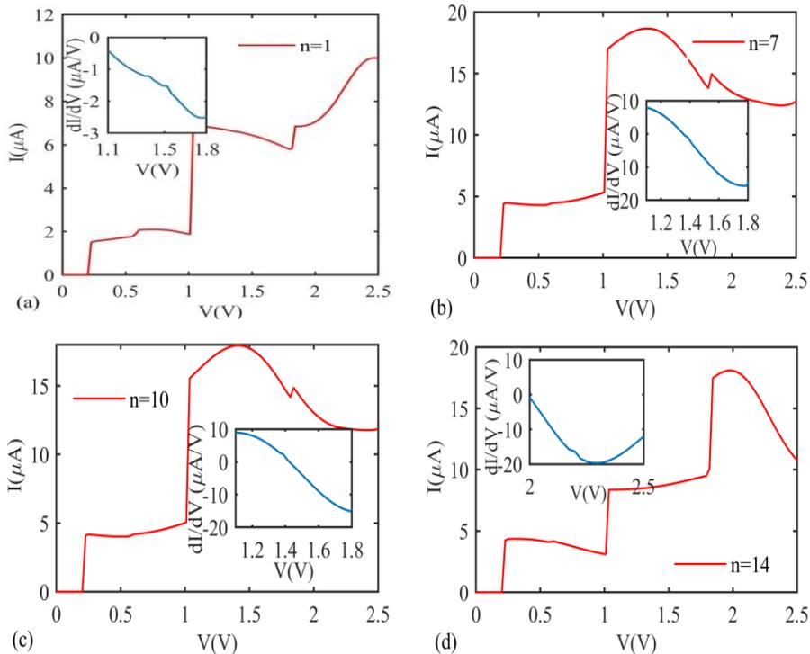
**Fig. 5.** (Colour on-line) I-V characteristics in the presence of impurity on (a)  $n=1,$  (b)  $n=7,$  (c)  $n=10,$  and (d)  $n=14.$  The insets show the differential resistance,  $dI/dV$  versus the bias voltage ( $V$ ).
