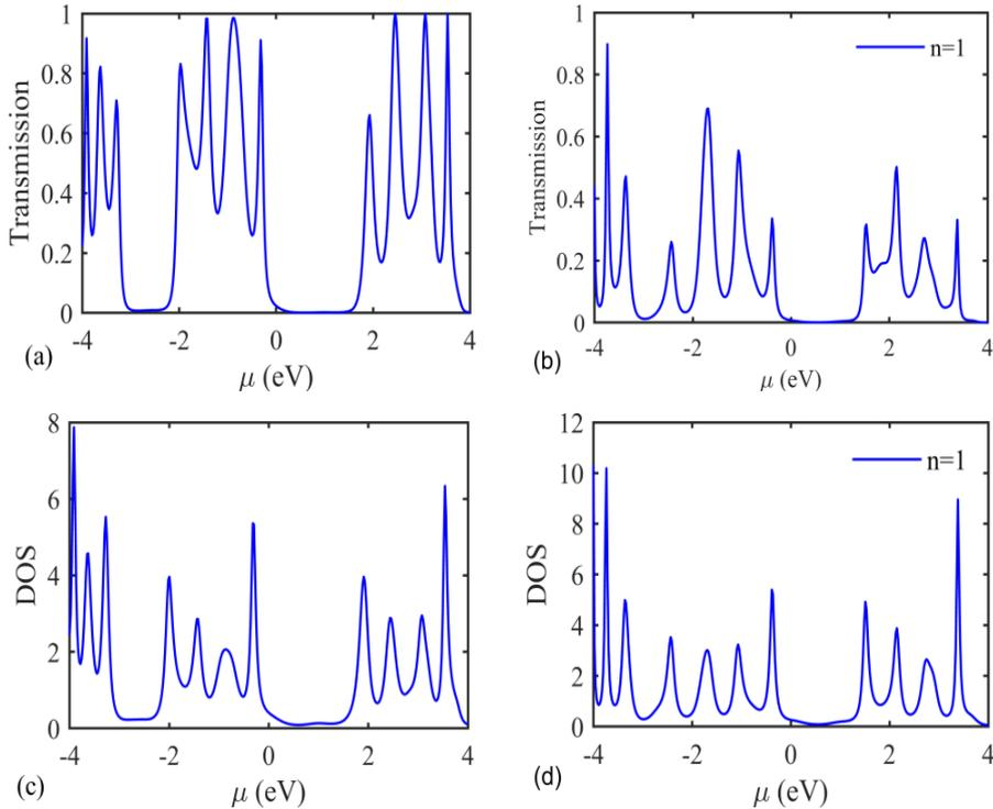
**Fig. 2.** Transmission function (a and b) and density of states of electrons (c and d) versus electrons energy (a and c) without impurity and (b and d) with impurity located on  $n=1$ .
