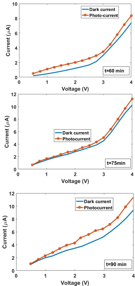
**Fig. 2.** I-V characteristics of thin MoS<sub>2</sub> films grown at different times for dark and illumination conditions. The bath temperature is held on T=60 °C.
