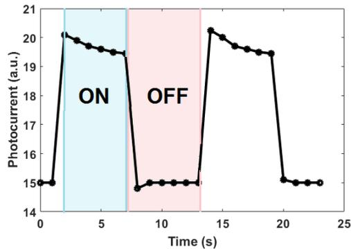
**Fig. 4.** Time response of grown  $\text{MoS}_2$  thin film to light source ON/OFF.
