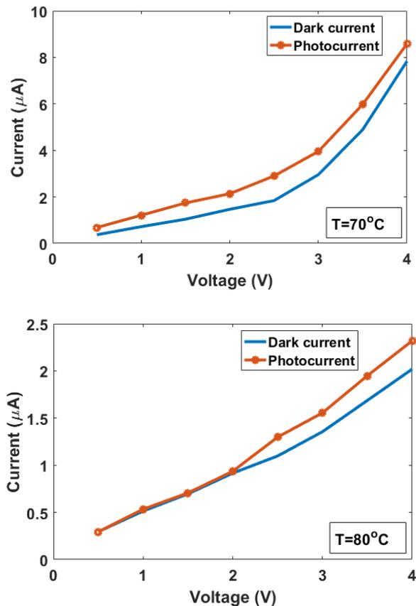
**Fig. 3.** I-V characteristics of thin MoS<sub>2</sub> films grown at different bath temperatures for dark and illumination conditions. The growth time is held on  $t=60$ min.
