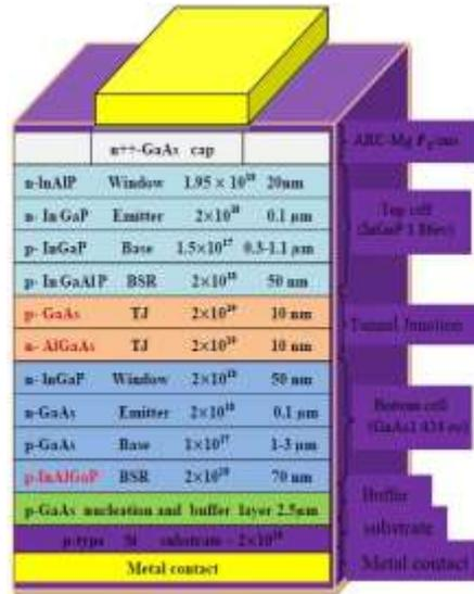
**Fig. 5.** The Structure of the proposed two-junction solar cell with a tunnel layer of (GaAs – Al GaAs) and Bsr (p-InAlGaP)
