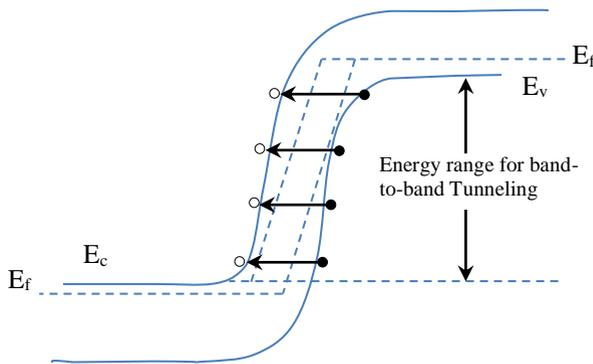
**Fig. 2.** Schematic band diagram of a tunnel junction.[34]
