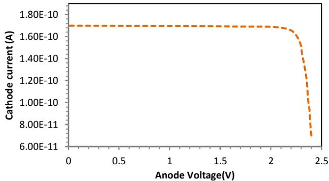
**Fig. 8.** Voltage current curve of the solar cell structure with tunnel layers of (GaAs – Al GaAs) and Bsr (p- InAlGaP)
