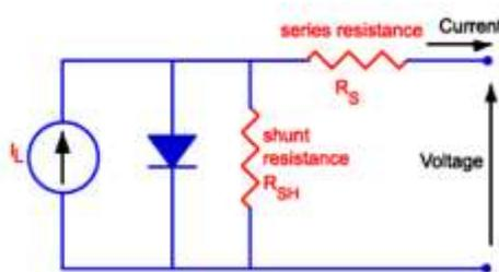
**Fig. 4.** The equivalent parasitic series and shunt resistances in a solar cell circuit
