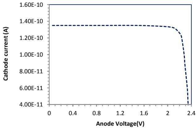
**Fig. 6.** Voltage current curve of the solar cell structure with Al GaAs – Al GaAs tunnel layer
