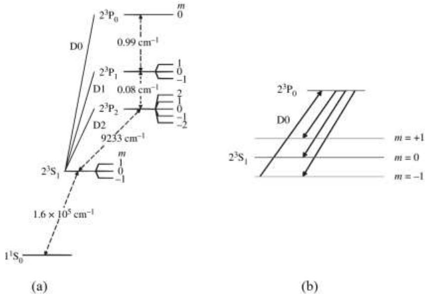
**Fig. 2.** a) Helium energy levels in an external magnetic field; b) Optical pumping of metastable atoms.
