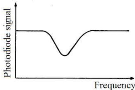
**Fig. 4.** Photodiode signal as a function of R.F. magnetic field frequency. The minimum point corresponds to the resonant frequency.
