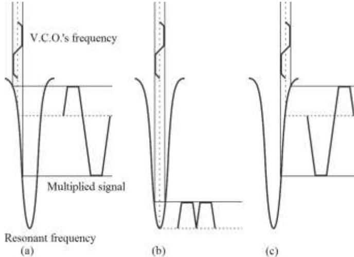
**Fig. 5.** The resonant and V.C.O.'s frequencies and their multiplied signal shape in different situations.
