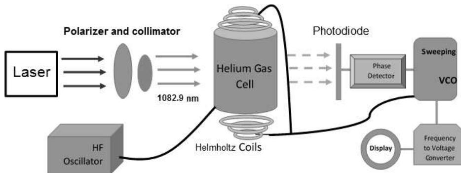
**Fig. 3.** A block diagram of a laser helium magnetometer.
