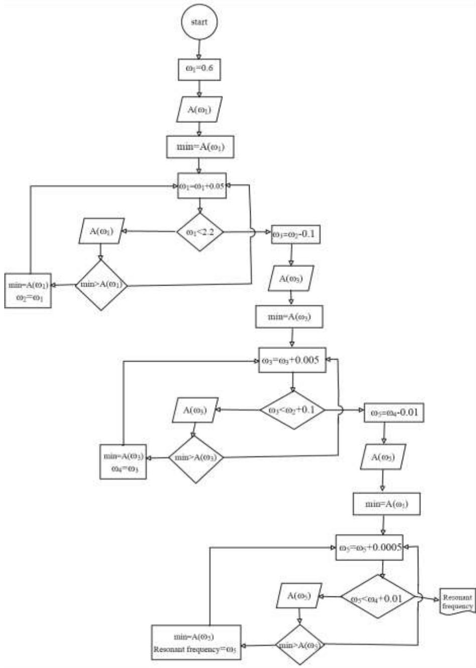
Fig. 6. The algorithm that is used in our calculation for conic method.
