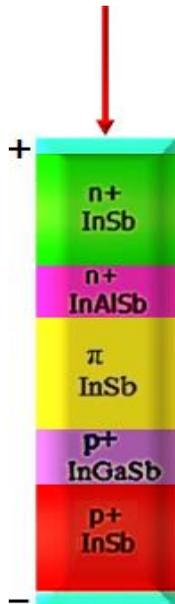
**Fig.3:** Schematic structure of the five-layer heterostructure
