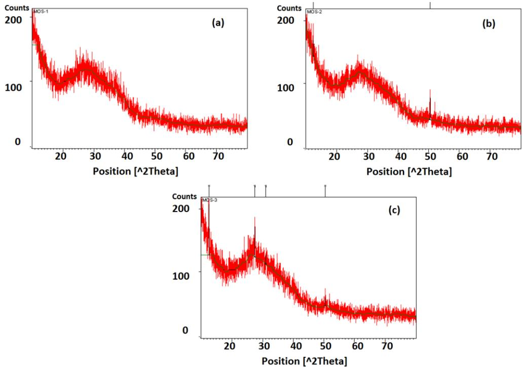
**Fig. 3.** XRD pattern for 3 samples grown in different conditions, (a)  $t=60\text{ min}$ ,  $T=30^{\circ}\text{C}$ , (b)  $t=60\text{ min}$ ,  $T=60^{\circ}\text{C}$ , (c)  $t=75\text{ min}$ ,  $T=60^{\circ}\text{C}$ .
