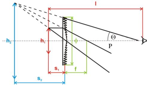
**Fig. 2.** A symbolic layout of Fresnel lens [8].
