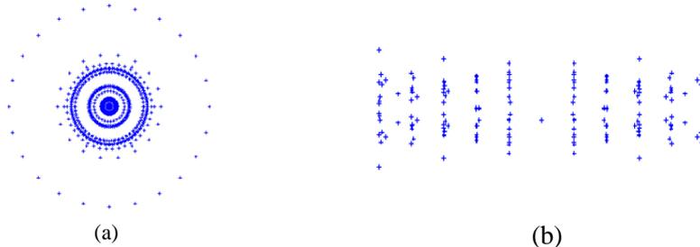
**Fig. 8.** (a) The stain obtained from the output rays in radial mode on the image plane after optimizing the Fresnel lens and (b) the stain obtained from the output rays in cylindrical mode on the image plane after optimizing the Fresnel lens.
