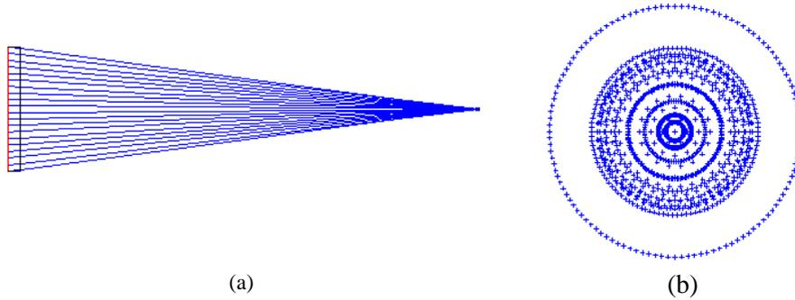
**Fig. 3.** (a) Simulation of Fresnel lens in sequential mode using Fresnel surface in Zemax software and (b) the stain obtained by the output rays on the image plane.
