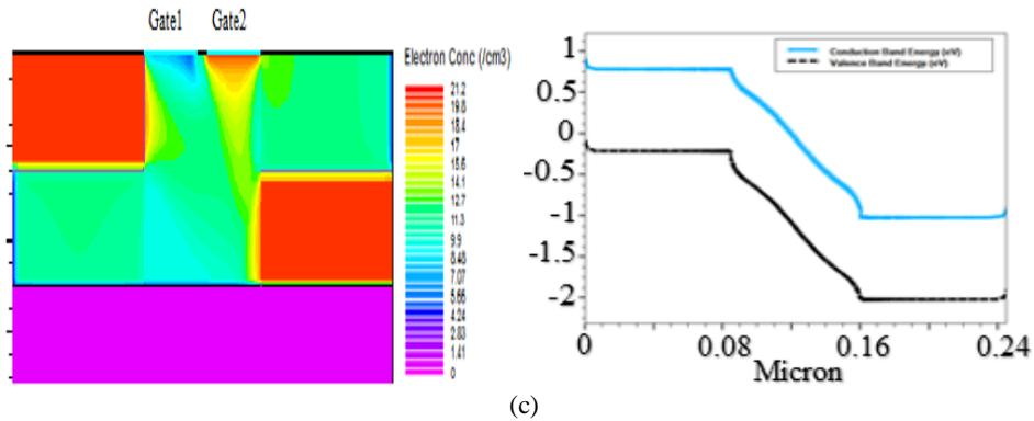
**Fig. 4.** Electron density and band diagram at a depth equal to 27 nm when the BTBT model is included in (a) the 35 nm channel length S-FED structure and (b) the 55 nm channel length S-FED structure (c) the 75 nm channel length S-FED structure.
