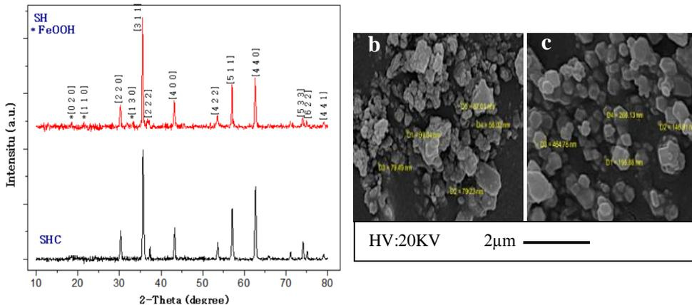
Fig. 1. a) XRD analysis of SH & SHC
