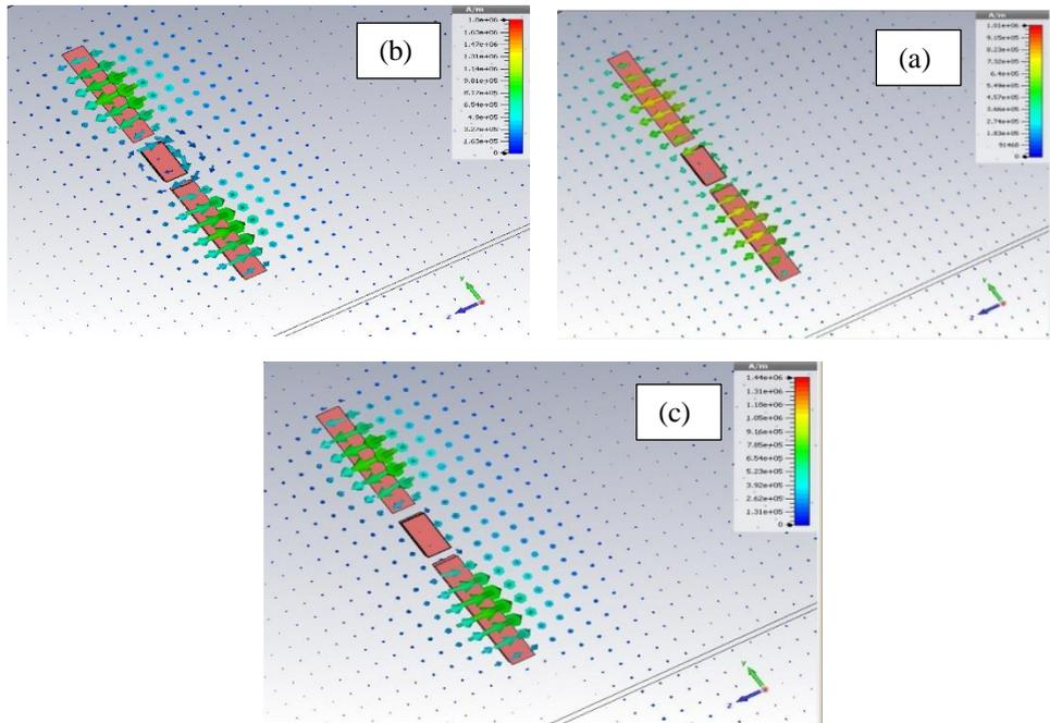
Fig. 5. Exhibition of the surface currents in bright and dark modes of the structure in a) 245 THz frequency, before resonance, b) 246.35 THz frequency, resonance frequency, c) 250 THz frequency, after resonance.
